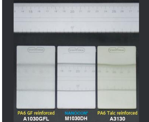
Surface appearance comparison of NANOCON® and conventional reinforced material
